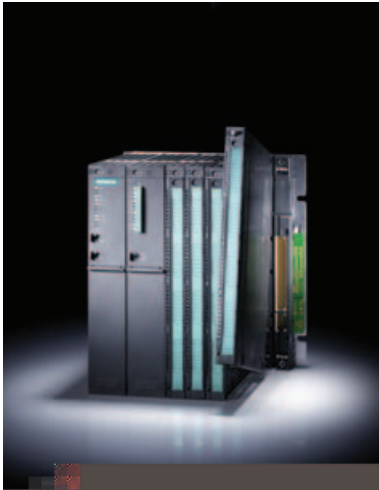
Easy assembly of S7-400 by hooking module into backplane
